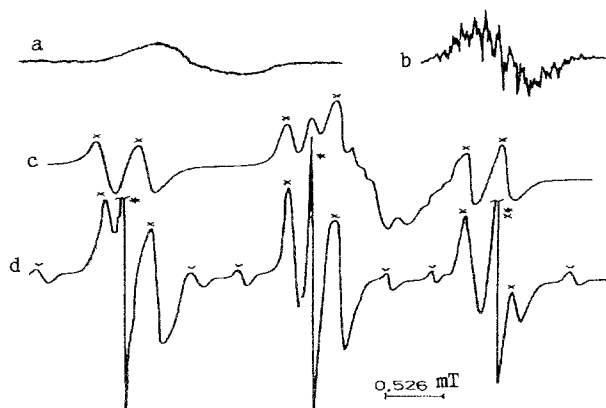
Fig. 1. EPR spectra observed during the vinylation of 2-phenylpyrrole: a) with phenylacetylene in the absence of the spin trap; b) with acetylene in the presence of the spin trap under high resolution (central portion of spectrum); c) with phenylacetylene in the presence of the spin trap 1 h after the start of the reaction; and d) after 3 h. Lines belonging to a single adduct are labeled with the same sign; *) di-tert-butyl-nitroxyl lines.
